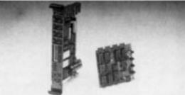
Being intelligent, this card eliminates all pots and manual adjustments. Everything is set up using a computeror dumb terminal like our Digital Audio Repeaters and Smart Brick Brains. Once programmed, the movementscan be burned into this card so that it can control four analog movementsall by itself. An optional LVDT (Linear Variable Displacement Transducer) signal conditioner is also available forthose who need it. This card should be available in production quantities by the end of the year.
