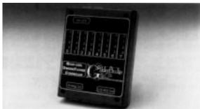
The Gildertluke and Company Quad-Level Dimmer and Flicker Controller can be used in a number of lighting applications with or without an Animation Control System. It controls up to eight lighting circuits simultaneously.
