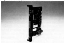
For expansion each Smart Analog Card features a connection for controlling Z-Bricks. These each feature thirty-two medium current outputs, and can be used just like a normal Smart Brick. The advantage Z-Bricks have is that, during programming, they can get their data from the DMX-512 input via the Smart Analog Card. Normal Smart Bricks require a temporary RTU/FSK unit or cables from the Digital Output Card in the PC·MACs system for programming.
