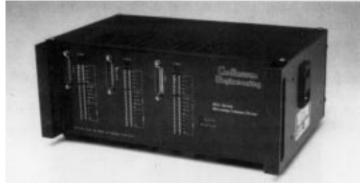
Rather than build high resolution servo and stepper motor controls ourselves, we are currently developing simple interfaces between PC·MACs and other manufacturer's motor controllers. The first of these is from Continuum Engineering. This is a self-contained micro stepping motor controller. Each unit can control up to three axis of motion, with up to 50,000 steps per revolution (based on a 1.8°, 200 step motor).
