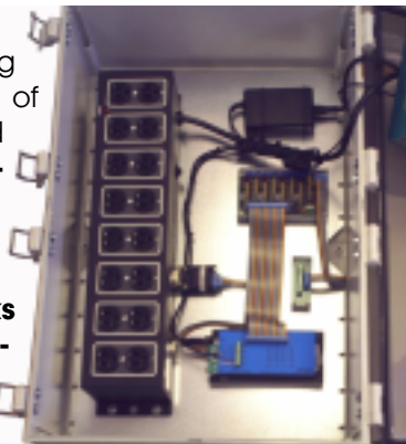
Distributed Fountain Controls w/ 8 115 VAC relays, 4 analog, Audio Playback
