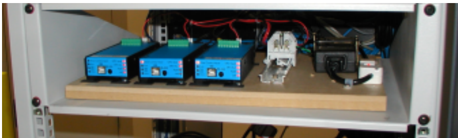
Distributed Show Control System using three Mp3-50/8s
