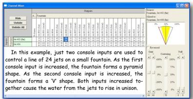
The final two Mixer controls are the 'null' sliders, these allow you to set an input so that it has no effect until it exceeds a minimum or maximum threshold. This is what is used in the lower eyelid example to keep the eyelids from moving down until the pupil starts looking upwards or downwards beyond a certain threshold.
