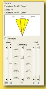
By shifting the 'centering', the output range is once again 0-100%, centered at 75%
