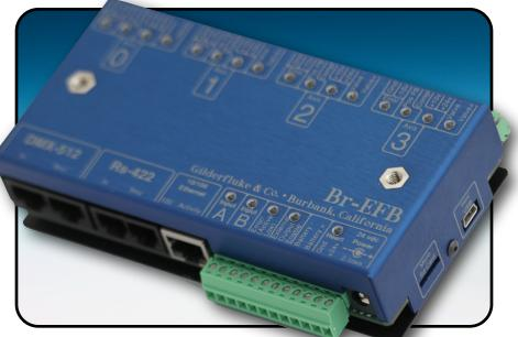
The **Br-EFB** is used when you need to close an analog servo loop used to control pneumatic, hydraulic or electric actuators. These are used in animated shows, motion bases, industrial systems, special effects, fountains, and more.
