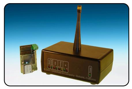
The **Bt-DMX** and **Bt-Servo** are used for wireless control of remote control-style Servo-Motors from a PC•MACs Animation Control System, Bs-Brain4, Sd-50 or any other source of DMX-512 data.
