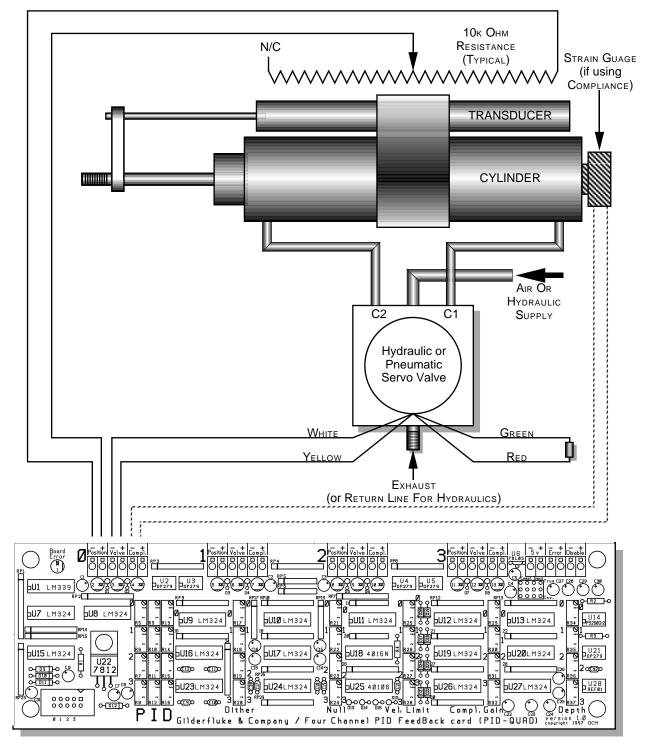
The cylinder can be virtually any type of double acting cylinder available (rotary, linear, etc.). The stroke and diameter of the cylinder can be used to determine the size of valve you need to use by
