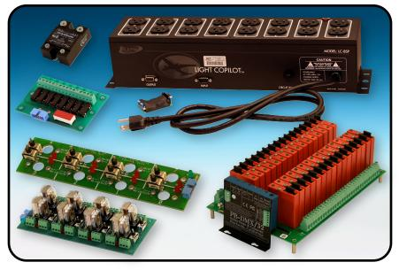
The outputs from Gilderfluke and Company's Animation Control Systems are designed to drive the majority of loads without relays. These 'relays' can be used where you need to control a higher current or voltage than the Animation Systems can provide directly, or when you need a completely isolated 'contact closure' output.
