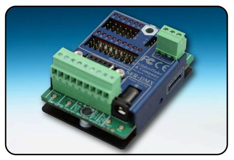
The **SER-DMX** is used for controlling remote control-style ServoMotors from its micro Sd card, or from any Gilderfluke Animation Control System or other DMX-512 source. ServoMotors are an inexpensive way to add analog movements to animated figures.
