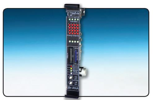
The **Br-ANA** is used when you need to control anything that needs a 0-10 vdc analog control voltage. These include animated shows, lighting, motion base simulators, pneumatic and hydraulic systems, special effects, signs, fountains, and more.
