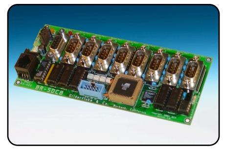
The **Br-SDC** is a complete, stand-alone Serial Output Controller. The **Br-SDC8** adds eight multiplexed RS-232 serial ports. It is used whenever you need to control eight devices that need strings of RS-232 serial data. It can be used to with nearly any RS-232 serial controlled devices. The **Br-SDC8** can be controlled from Gilderfluke & Co.'s Show Control Systems, PLCs or any other control systems. Just attach some buttons, and you can make your own interactive video kiosk.
