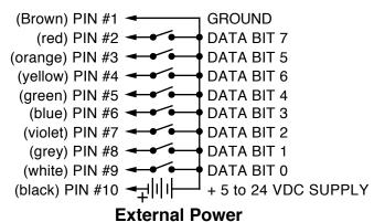
Any event can be triggered on either the 'closing' or 'opening' edge of any input. A 'closing' is when you ground an input. An 'opening' is when that grounding is removed. The inputs can be triggered on any voltage from 9 to 24 VDC. If you don't have an external source of power for these two inputs, you can 'steal' some juice from the **Br-SDC's** power supply.
