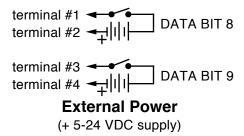
Versions of the **Br-SDC** 2.0 or later use a bipolar optoisolator on inputs 8 and 9. This means that you can ignore the polarity markings shown in the above illustrations on all versions of the **Br-SDC** 2.0 and later.
