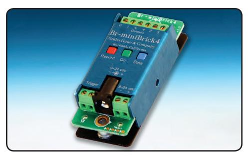
The **Br-miniBrick4** is a complete stand-alone Show Control System. It features a single 'trigger' input, and four high current outputs for driving solenoids, lights and relays.
