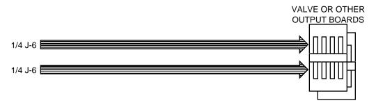
IF MORE THAN EIGHT OUTPUTS ARE NEEDED AT A GIVEN LOCATION, THEN MORE THAN ONE 1/4 J-6 CAN BE RUN TO THAT LOCATION.
