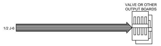
OR YOU CAN RUN A SINGLE 1/2 J-6 (20 CONDUCTORS), 3/4 J-6 (30 CONDUCTORS), OR FULL J-6 (40 CONDUCTORS) TO THAT LOCATION TO SUPPORT UP TO16, 24 OR 32 OUTPUTS AT THAT LOCATION.
