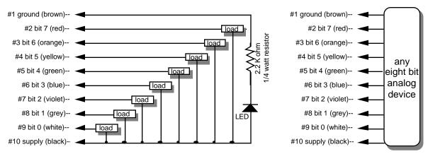
The supply line for each 1/4 J-6 is fused for 1 amp. You should treat each 1/4 J-6 as an individual, and not cross the outputs or supply lines from one channel to the lines from any other channel. Doing this won't cause any damage, but can reduce the protection for the outputs that the fuses normally provide.
