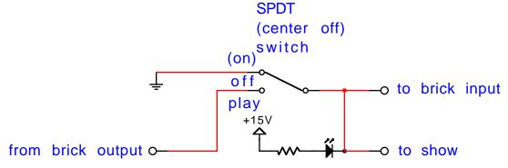
By adding a pushbutton switch to the connections shown above, you can make an easier to use programming console that has a separate 'programming enable' switch and pushbutton for turning on and off the output:
