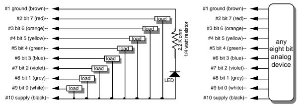
The supply line for each 1/4 J-6 is PTC fused for 1 amp. You should treat each 1/4 J-6 as an individual, and not cross the outputs or supply lines from one channel to the lines from any other channel. Doing this won't cause any damage, but can reduce the protection for the outputs that the fuses normally provide.
