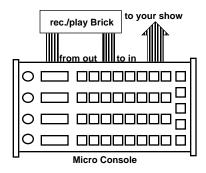
When building a programming console specific to your application, you can make it as simple or as complicated as you desire. Where a standard Micro Console can handle up to four 8 bit wide channels at one time, you can build your console to allow you to program just as many channels at a time as you want.
