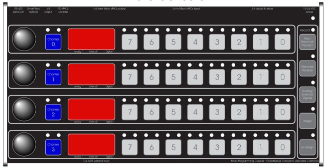
The Micro Console works with both PC·MACs and record/playback Brick Animation Control Systems. Up to four eight bit channels can be programmed at one time with the Micro Console. Each channel can be set to be used for eight digital inputs, the front panel eight bit resolution analog pots, or the external 0-10 VDC eight bit resolution analog inputs. A LED display shows the assignments and data on each channel.
