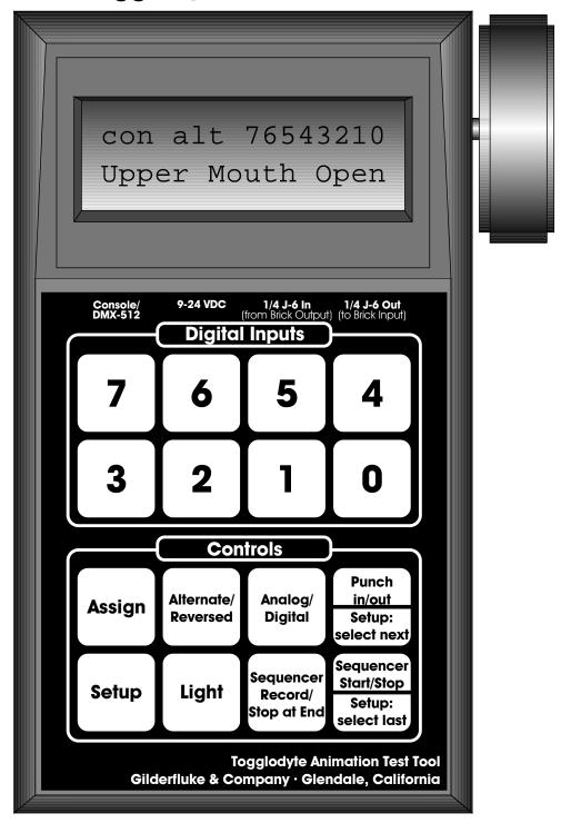
The Togglodyte is a small handheld unit which is typically used by service personnel to manipulate and move the animated figures that are attached to the Animation Control System. It can also be used as a simple programming console for generating animation data in real time.
