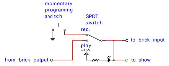
For building an analog programming console, we recommend you use our Analog to Digital (A/D) Converters. One is used for each analog function on your console. In this case the wires 'from brick output', 'to brick input', and 'to show' are actually eight wires (plus ground and + supply) that make up a 1/4 J-6 cable:
