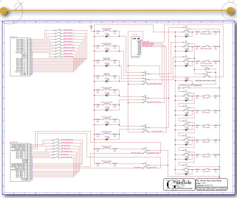
The other Safety inputs are wired to the KP-300's Error Inputs:
