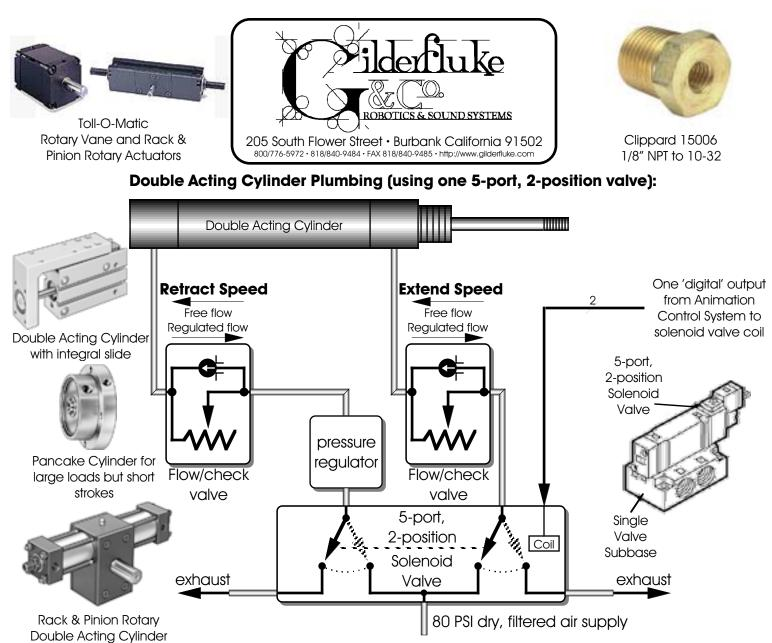
This is the way we recommend plumbing double acting cylinders if we don't need to stop them mid-stroke. It will allow the piston to be moved between the two extremes, and reversed smoothly mid-stroke when needed. Because you are regulating pressure flow out of the cylinder, this style of hookup usually will have a slightly better response time than traditional plumbing methods. The flow controls, which are a needle valve and check valve, don't interact when adjusted.
