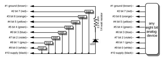
The supply line for each 1/4 J-6 is PTC fused for 1 amp. You should treat each 1/4 J-6 as an individual, and not cross the outputs or supply lines from one channel to the lines from any other channel. Doing this won't cause any damage, but can reduce the protection for the outputs that the fuses normally provide.
