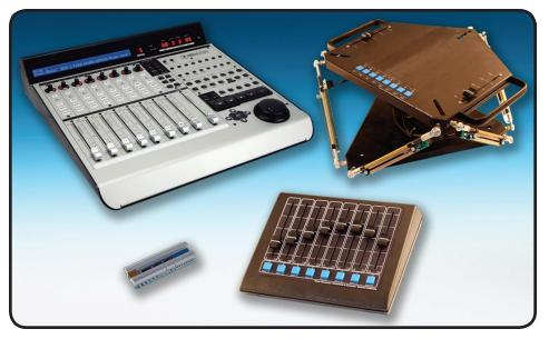
Programming Consoles are used to control the movements for an animated show in RealTime<sup>†</sup>. You move the controls, and **Pc•MACs** will remember exactly what you do.
