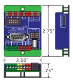
The **DAC-Quad** is used when you need to control anything that needs up to four 0-10 vdc analog outputs. These include animated shows, lighting, motion base simulators, pneumatic and hydraulic systems, special effects, signs, fountains, and more.
