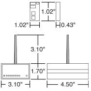
The **Bt-DMX** and **Bt-Servo** are used for wireless control of remote control-style ServoMotors from a **Pc•MACs** Animation Control System, **Br-Brain4**, **Sd-50** or any other source of DMX-512 data.
