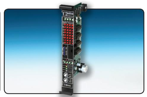
The **Z-Brick** is a complete thirty-two digital output Show Control System. The **Z-Brick** runs standalone, or as a 'master' or a 'slave' on a DMX-512 network. When running standalone or as a DMX-512 'master', it is just like a big **Br-MiniBrick8**, with four times the outputs and virtually unlimited memory capacity. It accepts data through its RS-422 or DMX-512 ports for RealTime programming, and stores shows on standard Sd/SdHC flash cards.
