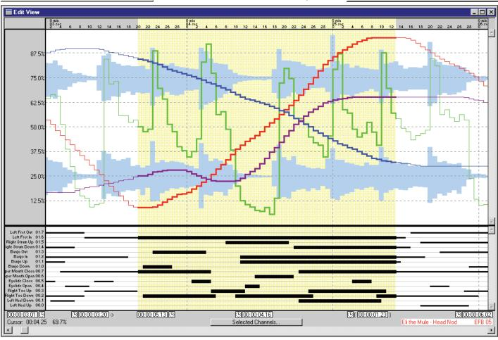
The OffLine editing screen lets you see and edit your show. Time scale is at the top. Analog moves and audio are in the upper window, digitals in the lower. If you are locking to a video, there will be a window to show that too. You can 'draw', smooth, cut, copy, paste, ramp, inbetween, fill, stretch, compress, reverse or invert movements. You can even program mouth moves by transferring the audio into them.
