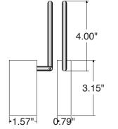
The **Linx-Rx** and **Linx-Tx5** or **Linx-Tx8** form an eight channel short range wireless link. The 1/4-J6 output from the **Linx-Rx** can be used directly to run small relays and solenoids, or fed into any of Gilderfluke's relay modules to control higher current/voltage loads. Most commonly, the output of the **Linx-Rx** is used to start a sound or show playing on a Gilderfluke audio repeater or show controller.
