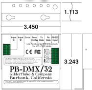
The **Pb-DMX/32** plugs right onto **Pb-8**, **Pb-16**, **Pb-24**, or **Pb-32** relay modules. The **Pb-DMX/32** receives DMX-512 data, RealTime serial data through its RS-232 serial port, or show data from its onboard data storage to control up to thirty-two AC or DC output relays. Using DMX-512 networking, 4096 relays can be controlled using just a pair of wires!
