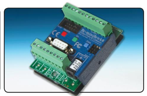
The **Br-miniBrick8** is a complete stand-alone Show Control System. It features two 'trigger' inputs, DMX-512 input or output, two airplane-style servo motor control outputs and eight high current outputs for driving solenoids, lights and relays.
