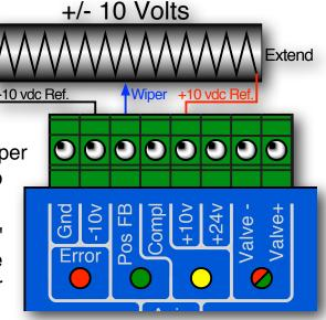
The Position Feedback Input (screw terminal position #3) is where you will normally connect the 'wiper' from a position sensing potentiometer. The retract end of the potentiometer would normally be connected to the
