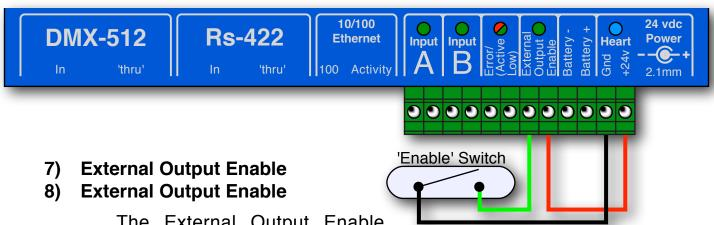
The External Output Enable Input will accept voltages from 5 vdc
