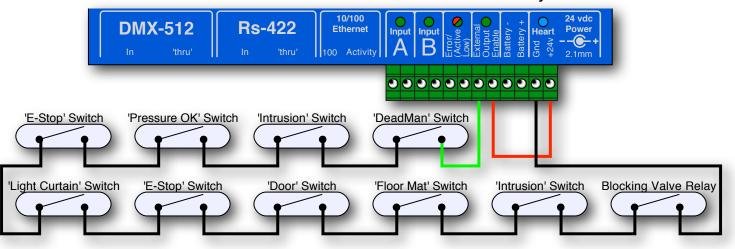
When the External Output Enable is asserted, the Br-EFB will do a long EaseIn on all enabled axis to keep the actuators from jumping. The Br-EFB will not signal an 'out of range' or 'following' error if the actuators are outside of their normal range of movement when the outputs are disabled, or during this initial EaseIn.
