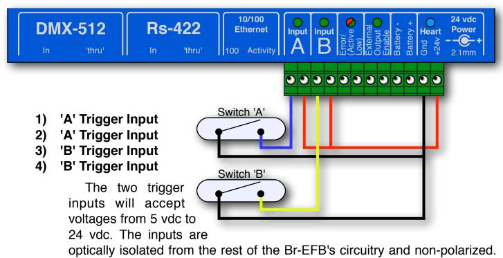
It is preferable (but not required) to provide an voltage from an external, isolated power supply. If you aren't using an isolated supply for these trigger inputs, you can borrow some power from the Br-EFB to power them, as shown in the illustration.
