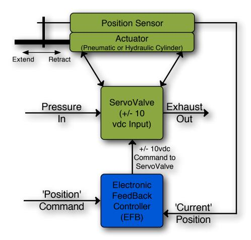
The complimentary outputs allows the Br-EFB to also work with non traditional ServoValves that want to see a unipolar outputs where five volts is 'stopped'. Voltages below five volts move the actuator in one direction, and voltages above five volts move the actuator in the other direction.
