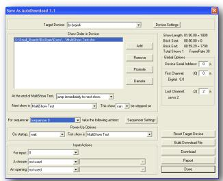
Pc•MACs uses the 'Target Device' to know what options are available for the Trigger Inputs, number of sequencers available, and even the size of the AutoDownload memory available. It looks this up from the GilderGearList each time you do an AutoDownload, so if new features have been added to the Br-EFB since your last AutoDownload, you will be able to access them.
