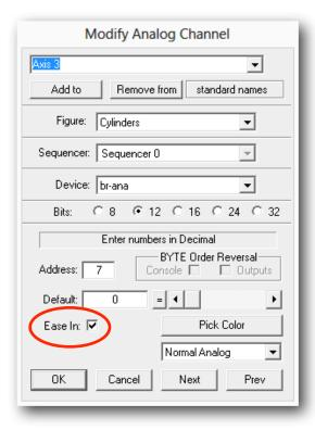
You can tell when an Ease-In is being performed by the Heartbeat flashing to twice normal speed. Once all outputs have dropped out of Ease-In mode, the heartbeat will return to its regular rate.
