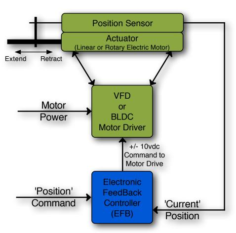
from your position and Compliance Feedback sensors. If you are using potentiometers, you will probably be using the Br-EFB's +/10 vdc reference outputs, and will set the inputs to match.
