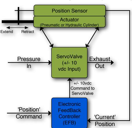
an external show control system, or from the AutoDownload file on the Br-EFB's  $\mu$ Sd flash card) with the actual position of the actuator (as measured by the position sensor). The EFB Controller will then open or close the ServoValve/Motor Controller a little or a lot (as needed) to send the actuator towards the requested position.
