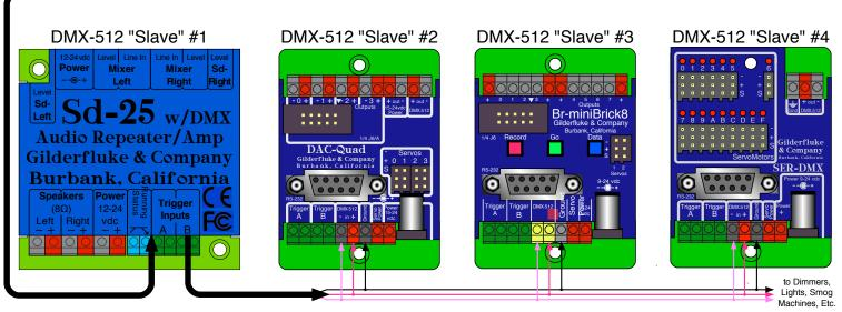
This illustration shows using a single Br-EFB as the 'DMX-512 'Master', and a Sd-25 w/DMX, DAC-Quad, Br-miniBrick8 and a SER-DMX as DMX-512 'Slaves'.
